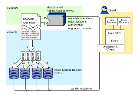
Figure 2.1: The XtreemFS architecture and components.
